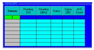
In this display you can see the status of all sensors currently connected to the computer.
