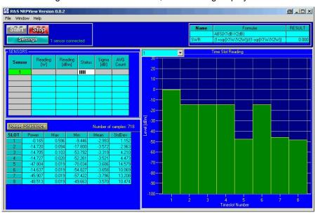
The drop down list at the top left of the timeslot display shows all sensors that are currently running in timeslot mode. You can select the one you want to see in the display and in the table.
