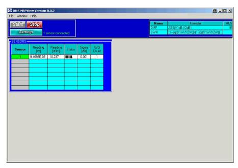
Now all connected sensors will run in their standard configuration in ContAv mode and display their results in the Sensors display.
