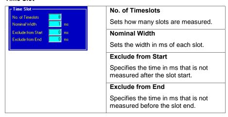
When running timeslot measurements, the following display is shown:
